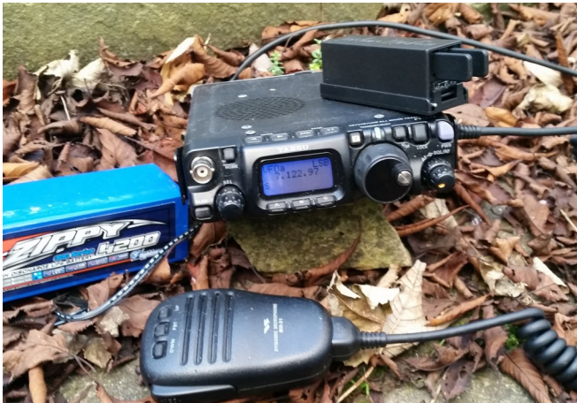
A typical HF setup: Portable radio, microphone, rechargeable battery, and Morse Code 'paddle'.
